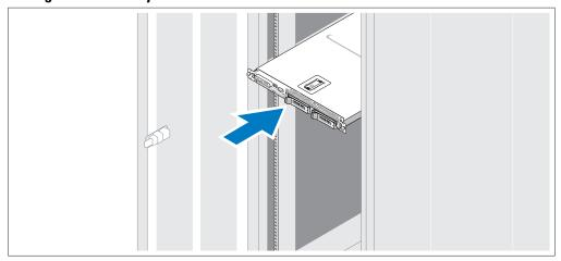
2 Install the system in the rack once you have read the "Safety Instructions" located in the rack installation documentation for your system.
