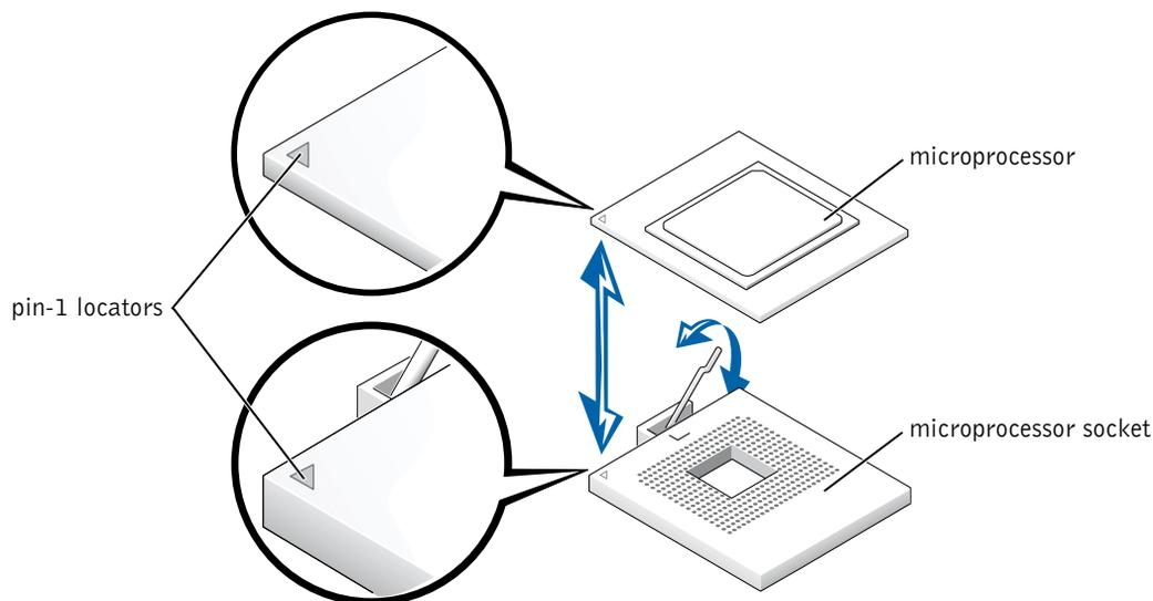
**NOTICE:** Positioning the microprocessor incorrectly can permanently damage the microprocessor and the system when you turn on the system. When placing the microprocessor in the ZIF socket, be sure that all of the pins on the microprocessor go into the corresponding holes. Be careful not to bend the pins.
