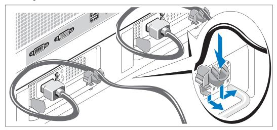
6 Attach the power cord retention bracket on the right bend of the power supply handle. Bend the system power cable into a loop as shown in the illustration and attach to the bracket's cable clasp. Repeat the procedure for the second power supply.
