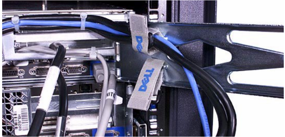
Figure 10. Securing the Power and CAT 5 Cables to the Cable Management Arm
