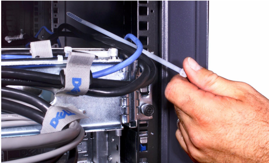
Figure 14. Securing the Power and CAT 5 Cables to the Rack
